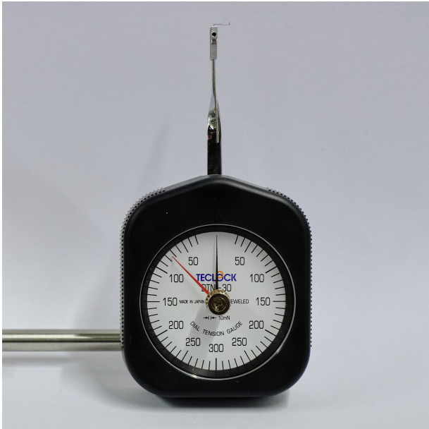
Figure 11: Federwaage des Pulltesters.
